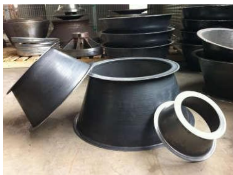
Housing of Diagonal Fan
