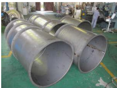
3mm Air Duct Flanging&Punching
