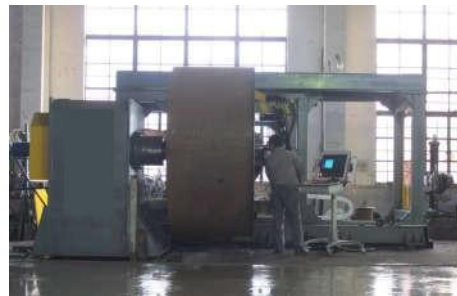
Okay FB2512 CNC Flanging & Punching machine
