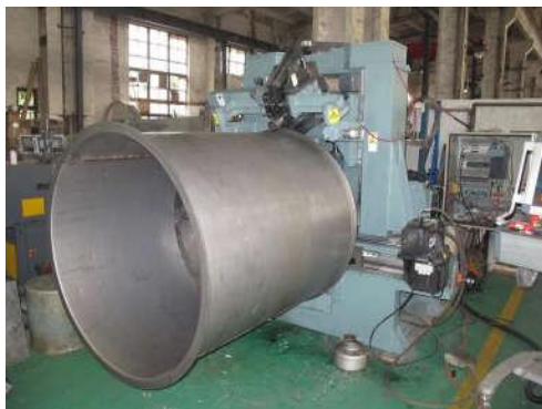
Fan Duct Flanging
